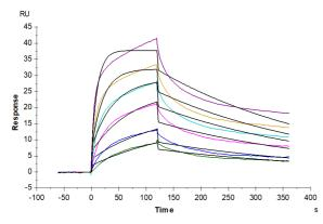
Biotinylated Human CCR6 Nanodisc, His Tag captured on CM5 Chip via Streptavidin can bind Anti-CCR6 Antibody, hFc Tag with an affinity constant of 3.57 nM as determined in SPR assay (Biacore T200).
